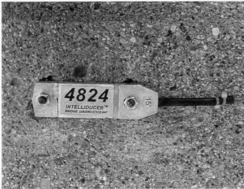
Figure 3.1. A BDI Intelliducer in use on top of a concrete curb.
